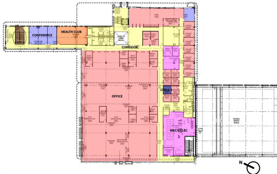
Figure 1-9-2: Second Floor Zones (AHU-2)
