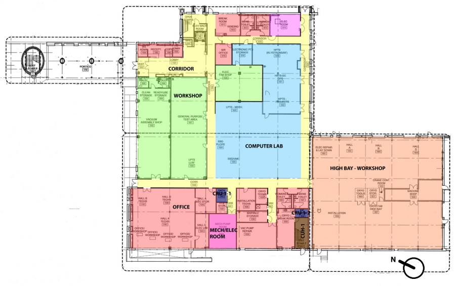
Figure 1-9-1: First Floor Zones (AHU-1)
